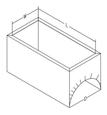
FLANGE-IN DESIGN: USED WHEN DIAMETER IS 2" OR GREATER THAN THE WIDTH.
