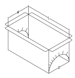
FLANGE-OUT DESIGN: USED WHEN DIAMETER IS THE SAME AS, OR LESS THAN 2" GREATER THAN, THE WIDTH.
