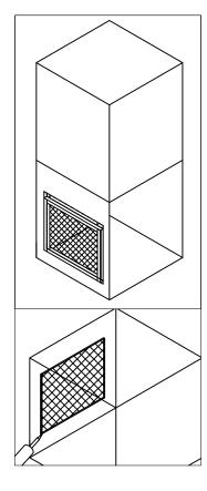
Step 2: Cut opening to accommodate filter rack (opening is 12 1/2" x 15 1/4" to fit side return kit). Space 4" from bottom and 3" from rear.
