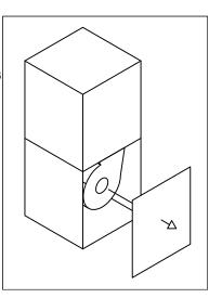
Step 3: Position the filter rack in the opening, and affix using six self-tapping sheet metal screws two on each flange (make sure to position the filter rack so the filter can slide in and out from the front). Apply sealant around interior border after installation (as shown). Make sure to apply to ALL FOUR SIDES for complete seal.
